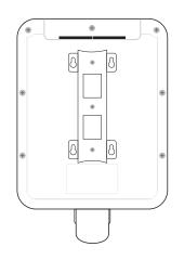
The back is composed of mounting brackets, which can be used for wall-mounting and pole-mounting.
